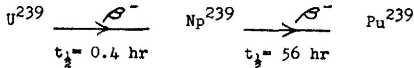
The decay of Np-239 takes place at approximately the same rate as decay of Pm-149 and it happens that the enrichment effect of the extra Pu-239 formed after shutdown almost balances the load due to Sm-149.
