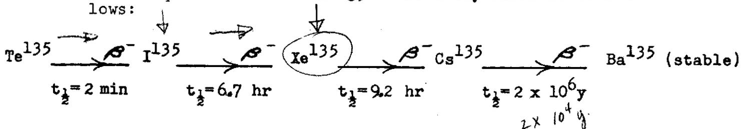
Xe-135 is removed from the reactor in two ways:
