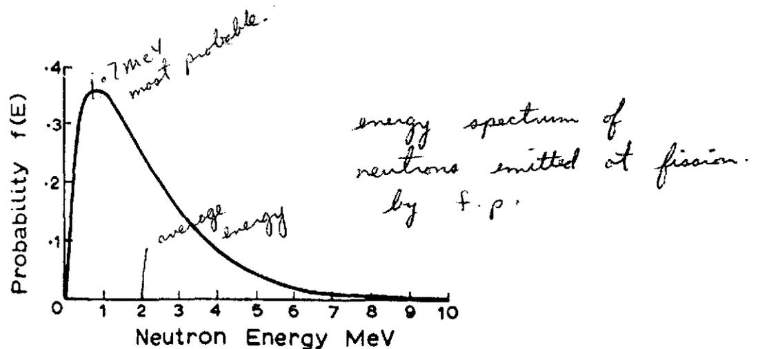
Fig. 3. Prompt Neutron Energy Spectrum
