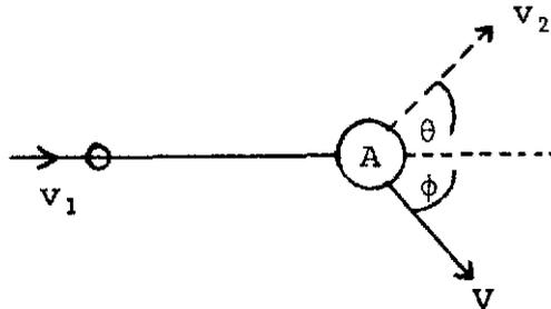
Fig. 3. Elastic Collision of Neutron with Moderator Nucleus
