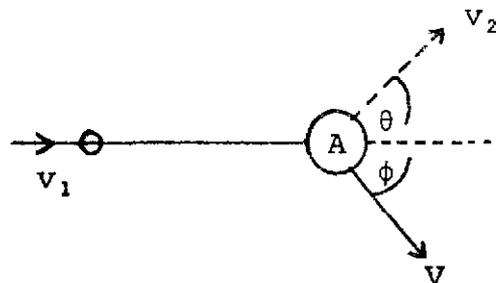
Fig. 1. Neutron Making an Elastic Collision
