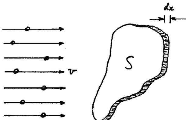
Fig. 1 Neutron Bombardment of a Thin Target
