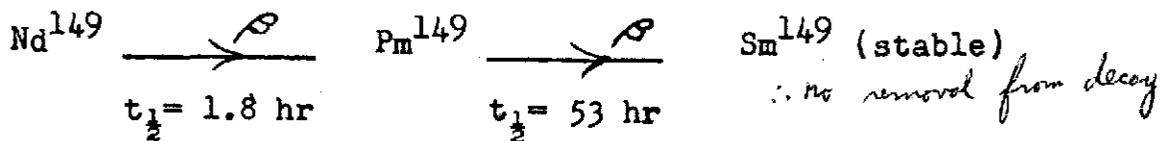
Sm-149 poison reaches its equilibrium in much the same way as Xe-135, as shown in the portion AB of the graph in Fig. 5. Sm-149, being stable, is not removed by decay and its rate of removal by neutron capture is slower than that of xenon. However, its rate of formation is also smaller, with the result that it reaches equilibrium more slowly than xenon. The Sm-149 equilibrium load is only slightly greater than a fifth of that of Xe-135.
